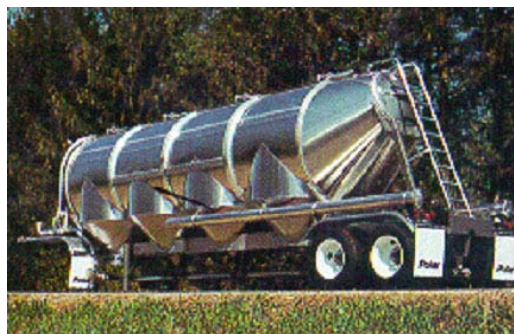
Figure 13(b): Tanks produced from bright rolled 5xxx alloy sheet.
