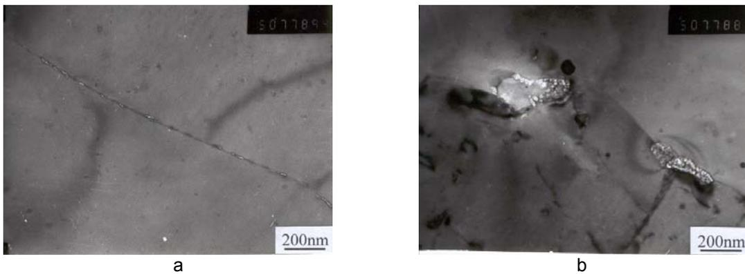
Figure 5: Superfine grain structures: a) uniformly located along a boundary (TX); b) generated as a result of accumulative recrystallization (TX+ 85°C, 2000 h)
