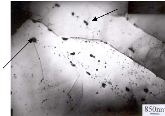
Figure 2: Recrystallized grain boundary, stable particles are noted with arrows, bright field (125°, 32 h).
