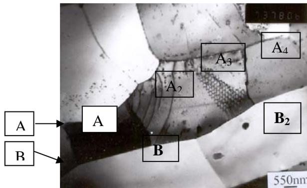
Figure 3: Bright field electron micrograph showing the structure of "subfibres".
