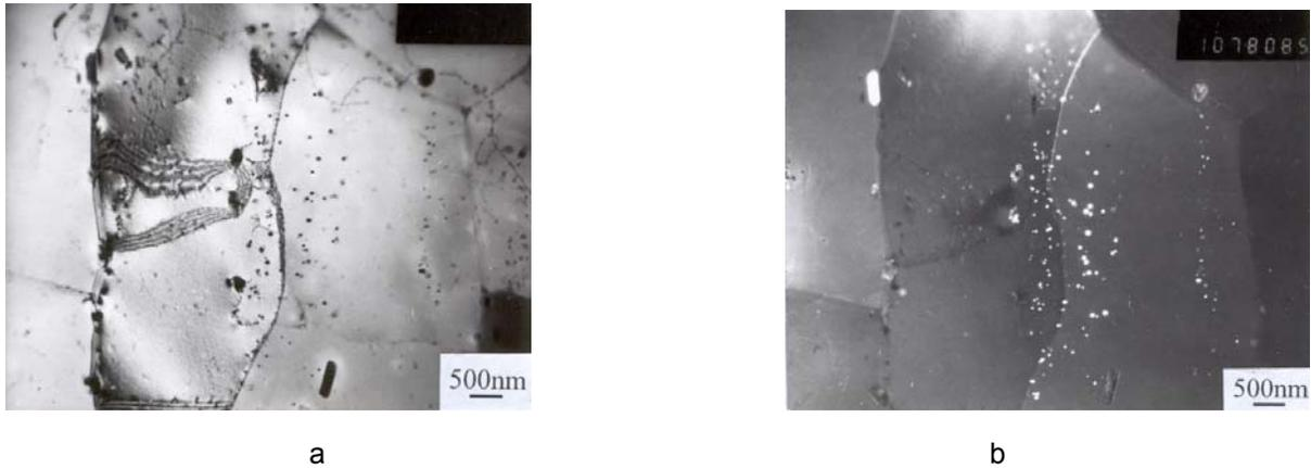
Figure 4: "Subfibre" boundary: a) bright field (125°C, 32 h), b) dark field using  $\delta'$ -phase diffracted spot.
