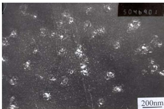
Figure 6: Weak beam (g; 3g ) revealing dislocation structure around  $\delta_{\text{non}}$ - precipitates (150°C, 32 h).
