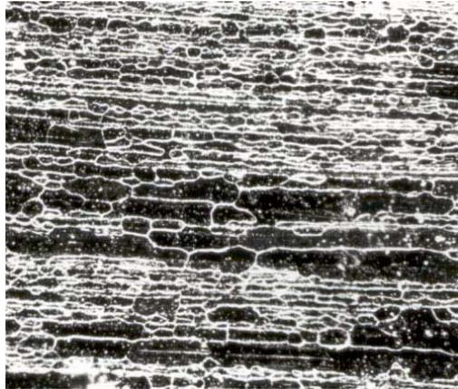
Figure 1: Microstructure of 1424TG1 Alloy (125°C, 32 h)
