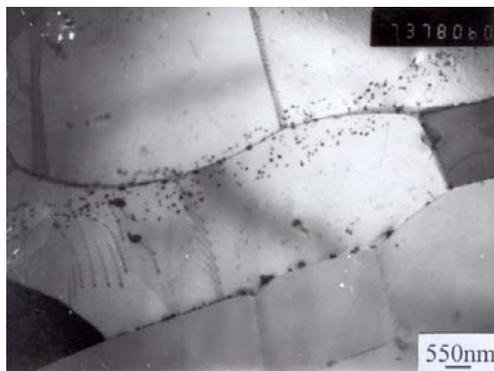
Figure 8: Stripe of  $\delta_{\text{non}}$ -phase particles accumulation along a "subfibre" boundary, bright field (125°C, 32 h).
