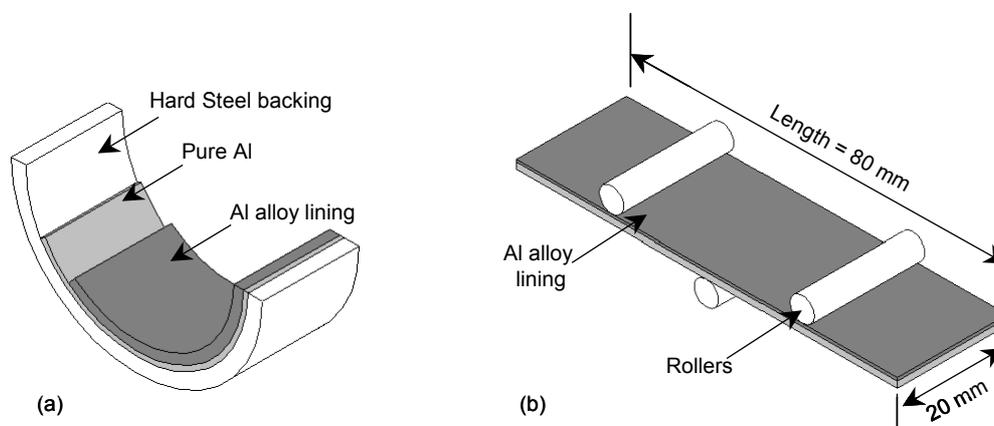
Figure 1: Schematic representation of (a) bearing geometry and (b) flat-strip fatigue set-up.
