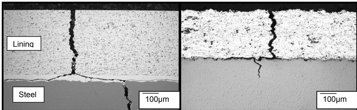
Figure 5: (a) Crack deflection perpendicular to the interface along the softer Al interlayer in RB lining system (b) Crack deflection along the interface in the HVOF lining. Note porosity in HVOF coating
