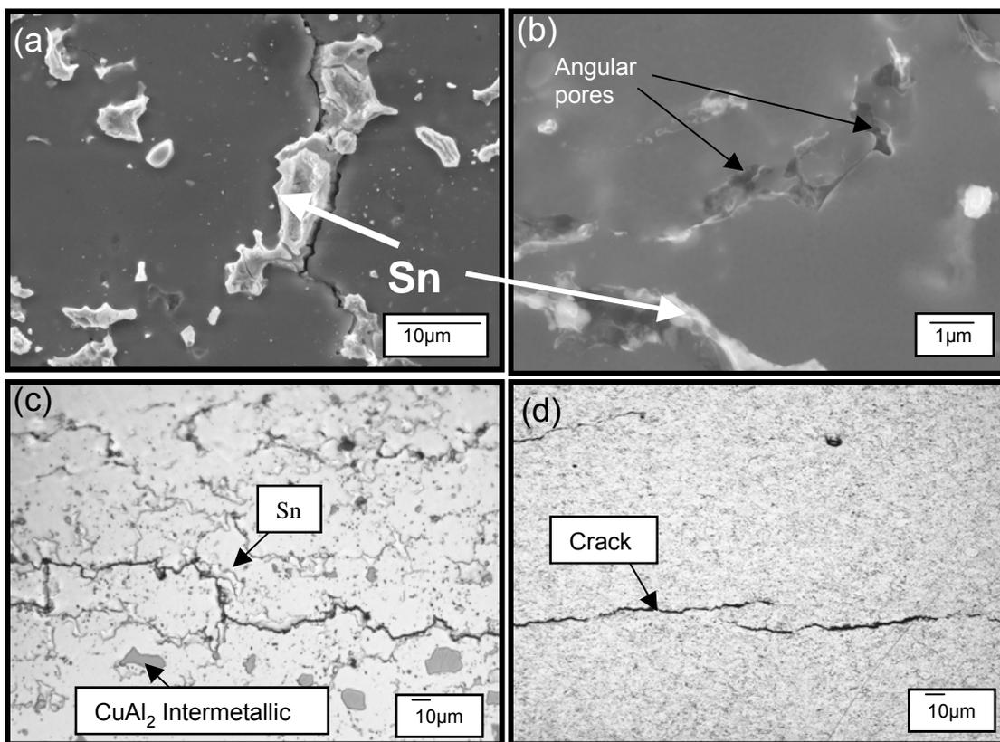
Figure 4: (a) RB lining, fatigue initiation observed by decohesion at large Sn particles (b) porosity observed in HVOF lining and very occasional large Sn particles (c) crack propagation in RB lining, note deviation of crack along the Sn-matrix interface (d) crack propagation in HVOF lining
