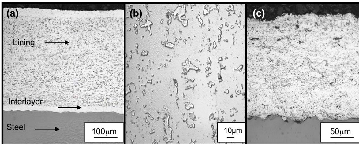
Figure 2: Polished sections showing (a) RB lining and steel backing (b) higher magnification view of the RB lining material (c) HVOF lining and steel backing, note rougher interface c.f. RB lining system.
