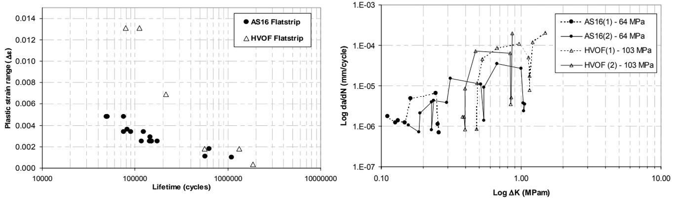
Figure 3: (a) HVOF and RB (labelled AS16) fatigue life-time comparisons in terms of estimated plastic strain range (b) crack growth rate comparisons in HVOF and RB linings. Note the difference in nominal maximum stress levels (64MPa for RB lining compared with 103 MPa for HVOF lining).
