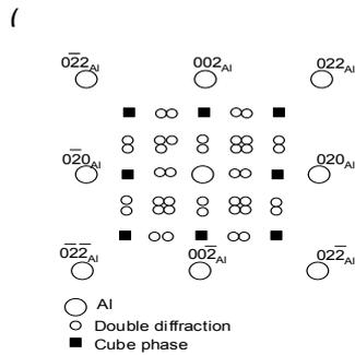
Figure 2: (a) SADP taken from the cube-shaped phase and (b) its schematic diagram.
