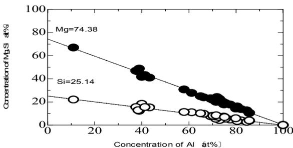
Figure 3: Extrapolation plot for EDS analysis.
