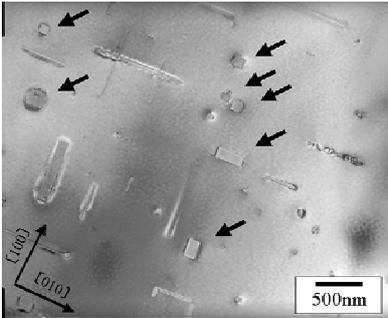
Figure 1: TEM image for A1.0mass%Mg<sub>2</sub>Si-0.4mass%Mg aged at 623K for 6ks.
