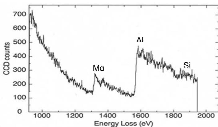
Figure 5: EELS spectrum taken from cube shaped phase.
