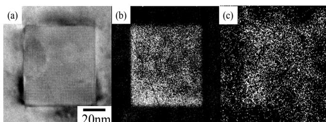
Figure 4: EFTEM images of cube-shaped phase (a) zero-loss image and (b) Mg-K map (c) Si-K map.
