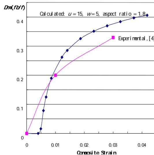
Figure 1: Calculated and measured damage evolution of the (SiC)p/Al-2618 composite at room temperature.
