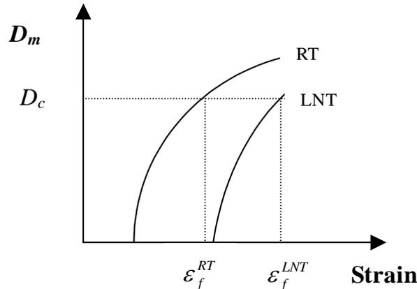
Figure 3: Schematic showing the effect of cryogenic temperature on ductility of a particulate composite.
