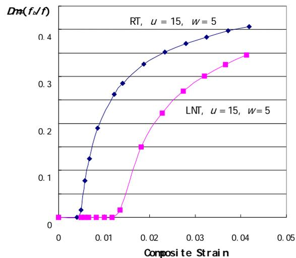
Figure 2: Calculated damage evolution of the (SiC)p/Al-2618 composite at room and liquid nitrogen temperatures (aspect ratio =1.8).
