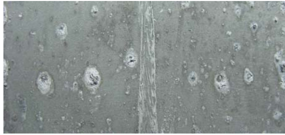
Figure 2: Corrosion appearance of a 2024T3 specimen. ( T=25^{\circ}\text{C} , \text{RH}=55\% , [\text{Cl}]=5\% [\text{SO}_4^{2-}]=5\% )
