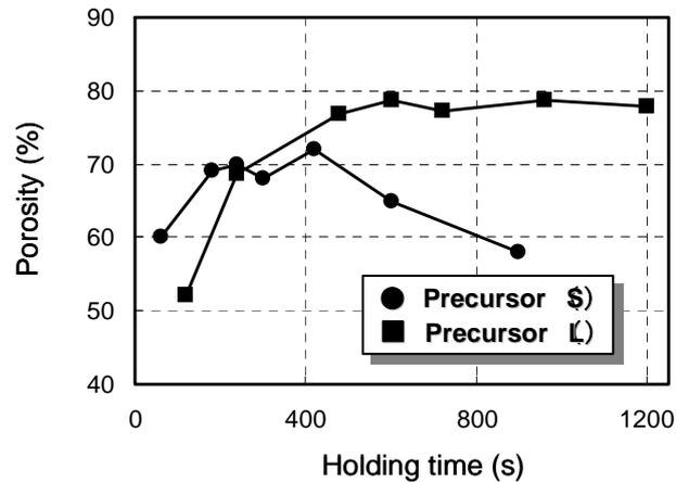
Figure 8: Porosity of the precursors (S) and (L).
