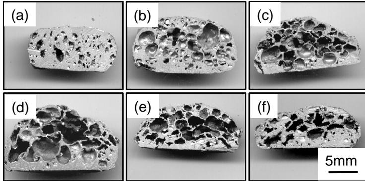
Figure 5: Cross sections of porous Al (pure Al/TiH<sub>2</sub> precursor), Holding Time (a) 60s, (b) 180s, (c) 300s, (d) 420s, (e) 600s, (f) 900s, (Holding Temperature: 973K)
