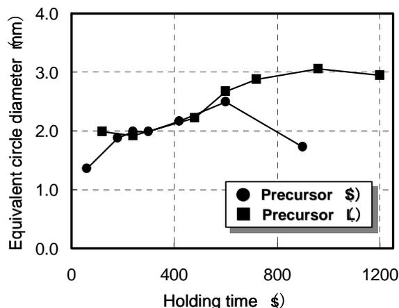
Figure 9: Mean size of the pores of precursors (S) and (L).
