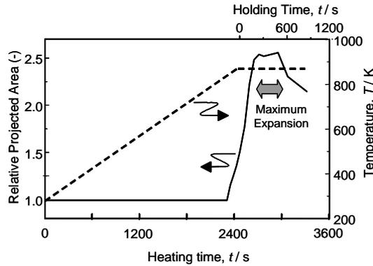
Figure 2: Relative projected area of Al-7Si/TiH<sub>2</sub> precursor (Holding Temperature: 883K).
