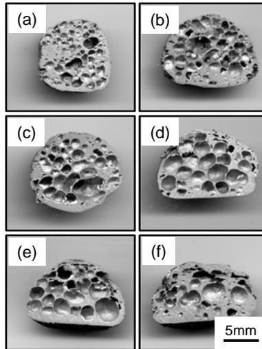
Figure 3: Cross sections of porous Al (Al-7Si/TiH<sub>2</sub> precursor), Holding Time (a) 60s, (b) 180s, (c) 300s, (d) 420s, (e) 600s, (f) 900s (Holding Temperature 883K).
