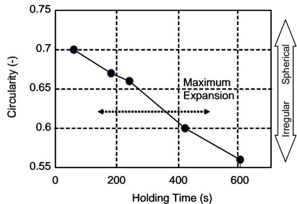
Figure 7: Circularity of pores of Al-7Si/TiH<sub>2</sub> precursor during holding process (Holding Temperature: 973K).
