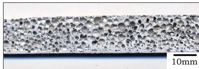
Figure 11: Cross-section of Al foam fabricated by powder processing technique.
