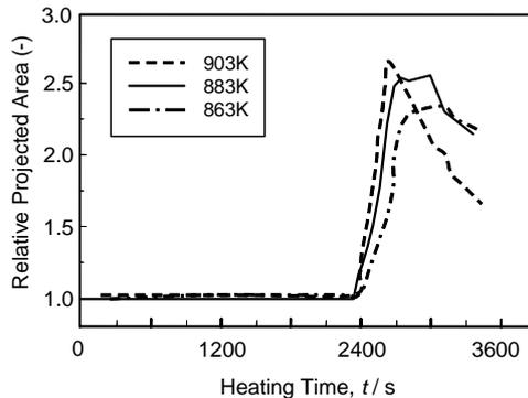
Figure 4: Relative projected area of Al-7Si/TiH<sub>2</sub> precursor (Holding Temperatures: 863-903K).
