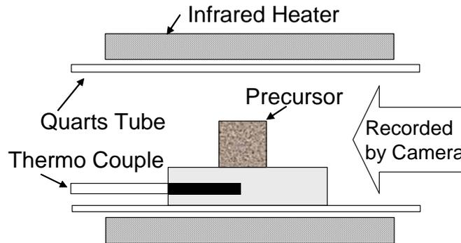
Figure 1: Schematic illustration of the experimental apparatus.
