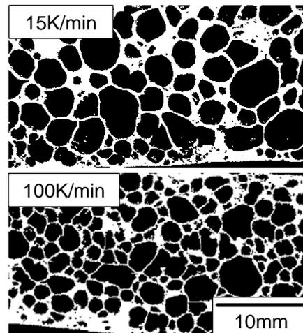
Figure 10: Black and white images of the cross-section of aluminum foams fabricated by different heating rates
