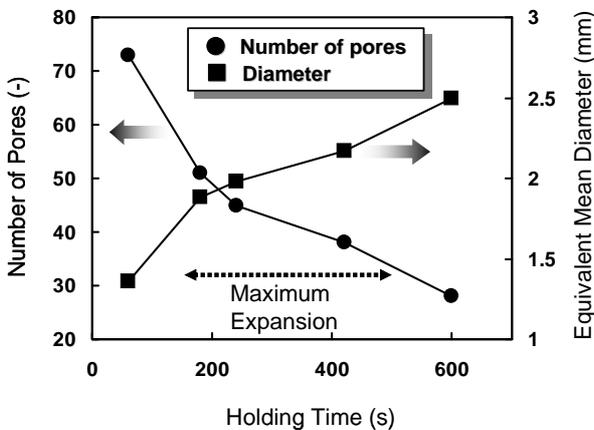
Figure 6: Number and mean size of pores of Al-7Si/TiH<sub>2</sub> precursor at different holding temperatures.
