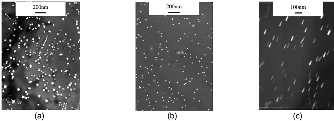
Figure 2: Dark field TEM-images of alloy 1 showing a) small, faceted Mn-bearing phases after slow heating (50°C/h) to 450°C, b) an area with a high Al<sub>3</sub>Zr number density after 12 hours annealing at 450°C and c) colony of AlZrSi-phases after 36 hours annealing at 450°C.
