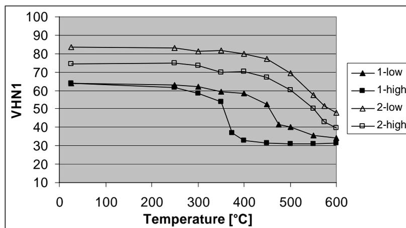
Figure 5: Isochronal softening curves (1/2 hr. at temperature) for both slowly heated (50°C/h) and rapidly heated (salt bath) variants of alloys 1 and 2.
