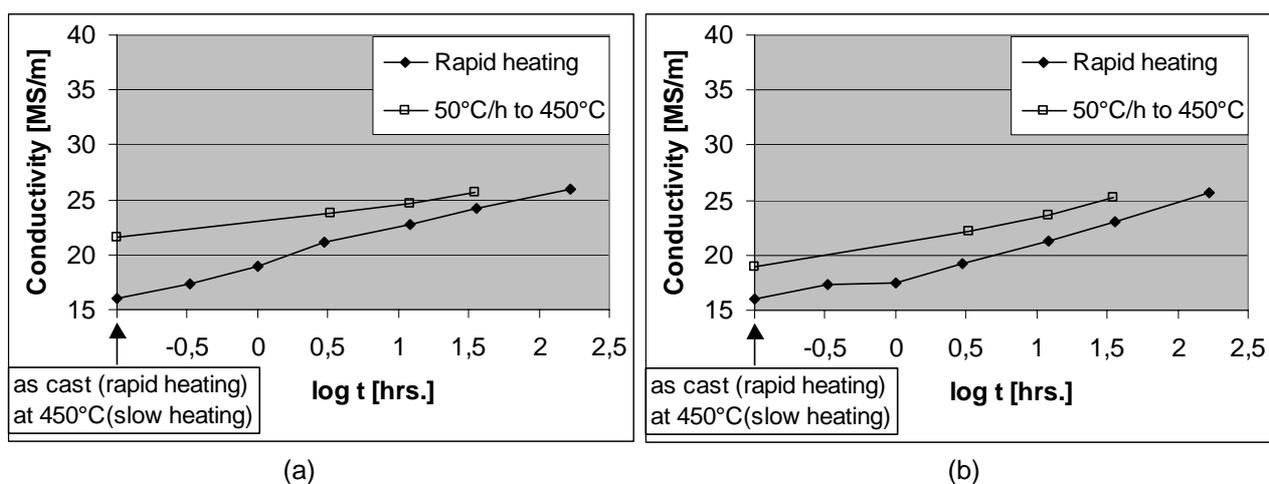
Figure 1: The evolution in conductivity for both variants of a) alloy 1 and b) alloy 2 during annealing at  $450^\circ\text{C}$ . The text boxes and arrows indicate where the values measured in the as cast material and after slow heating ( $50^\circ\text{C/h}$ ) to  $450^\circ\text{C}$  can be found.
