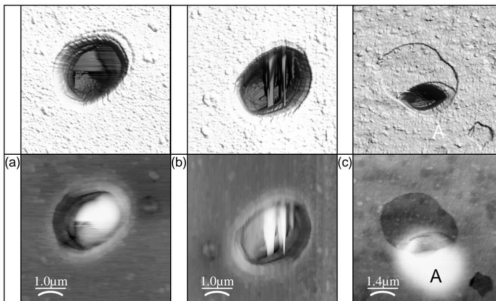
Figure 3: SKPFM height (top) and potential (bottom) images: (a) Pit after 5 min immersion,  $0^\circ$  scan angle, (b) Pit after 5 min immersion,  $90^\circ$  scan angle, (c) Pit after 10 min immersion.
