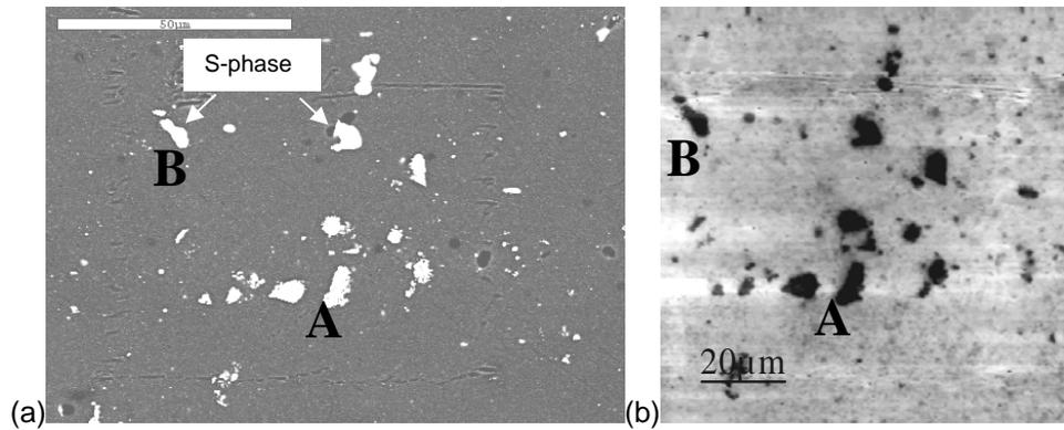
Figure 1: Characterisations of polished 2024 with (a) Backscattered SEM and (b) SKPFM potential image.
