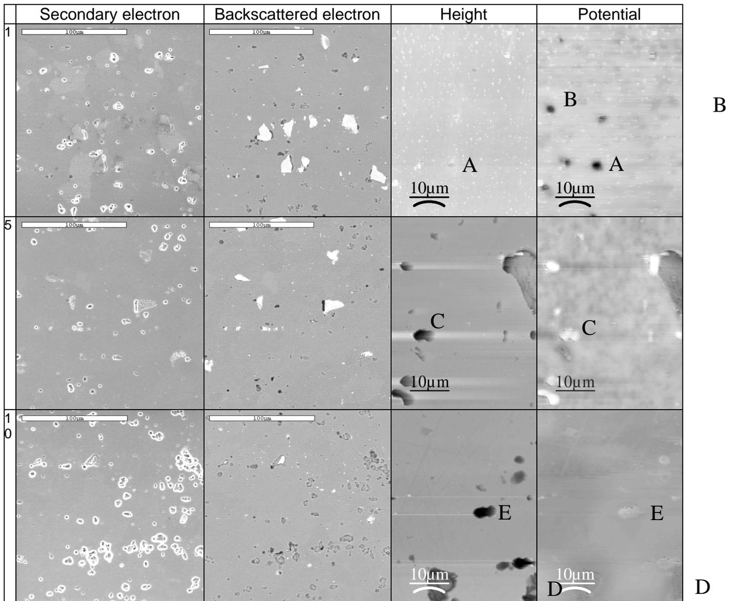
Figure 2: SEM and AFM-SKPFM characterizations of polished 2024 after 1, 5 and 10 minutes deoxidation.
