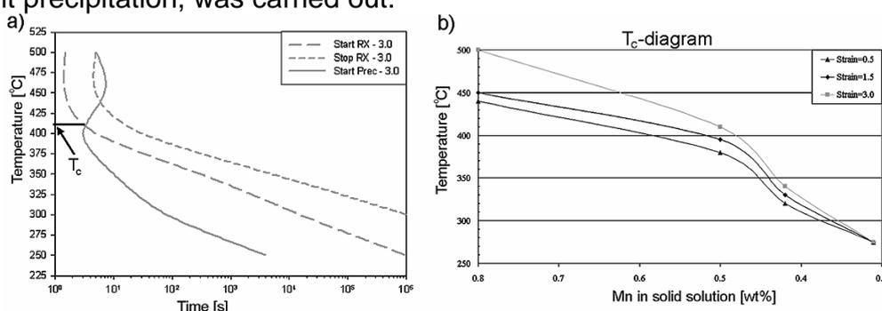
Figure 1: a) TTT-diagram of material A deformed to a strain of 3.0 and subsequently annealed at different temperatures. b)  $T_c$ -diagram of the different material conditions.
