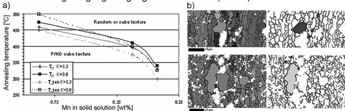
Figure 3: a)  $T_C$ -diagram and indication of at which temperature a change in recrystallisation texture is observed. b) OIM-maps of an annealed A-condition. Left figures show the raw map, including all grain boundaries, white areas are unindexed regions, most probably particles. Right figures show the grain boundaries and some shaded recrystallised grains comprising the P and ND-rotated cube orientations.
