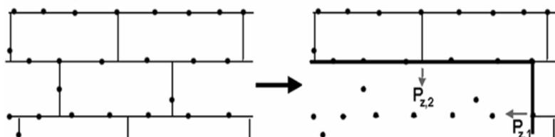
Figure 5: Schematic illustration of the effect of precipitation on recrystallisation. Thin lines are substructured regions, while thick lines represent migrating HAGB and dots are precipitates.
