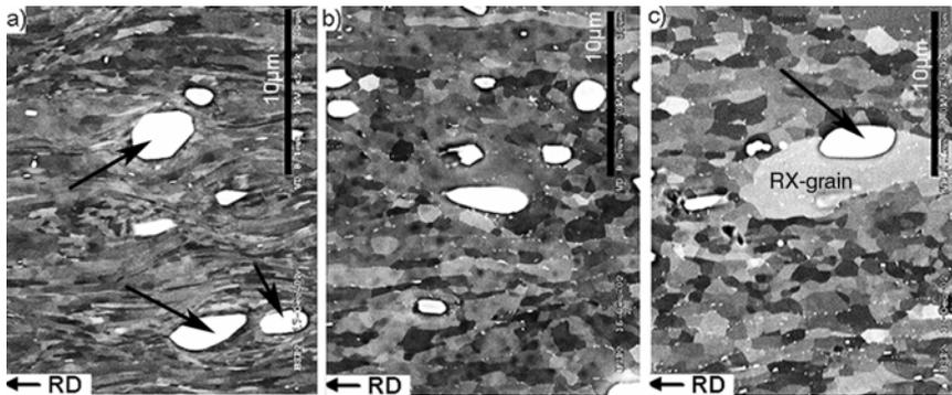
Figure 4: Microstructural evolution of the A-material a) deformed b) annealed 60s at 350°C and c) 10 min
