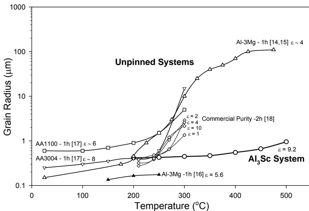
Figure 6: Grain radius as a function of annealing temperature (1h and 2h annealing at a given temperature) for Al-0.2Sc and various commercial Al alloys produced by ECAP.
