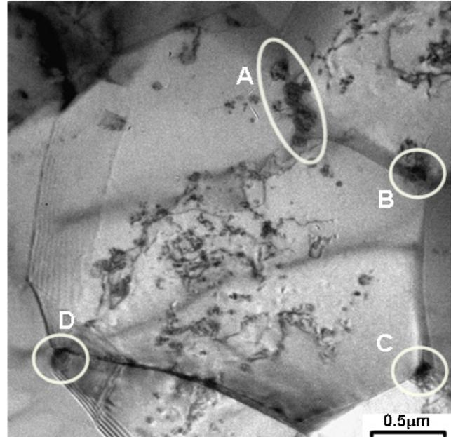
Figure 5: Al-0.2Sc pre-aged for 3h at 350°C and annealed for 1h at 500 °C. Particle pinning is evident at point A (4 particles) as well as B, C and D (1 particle each at triple points).
