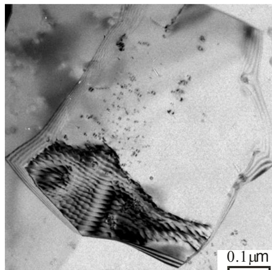
Figure 1: (a) Series of Bright field TEM micrographs at various tilt angles and the SAED pattern of a representative region of microstructure after pre-ageing for 3h at 350 °C (samples sectioned perpendicular to extrusion axis, ED). (b) Bright field TEM micrograph of microstructure after pre-ageing for 3h at 350 °C showing fine coherent  $\text{Al}_3\text{Sc}$  particles within a recovered grain and slightly coarser particles on grain boundaries.
