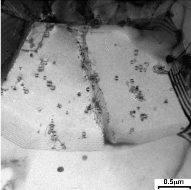
Figure 4: Al-0.2Sc pre-aged for 3h at 350°C and annealed for 2h at 500 °C showing coherent particles within a recovered grain and coarser particles interacting with grain boundaries.
