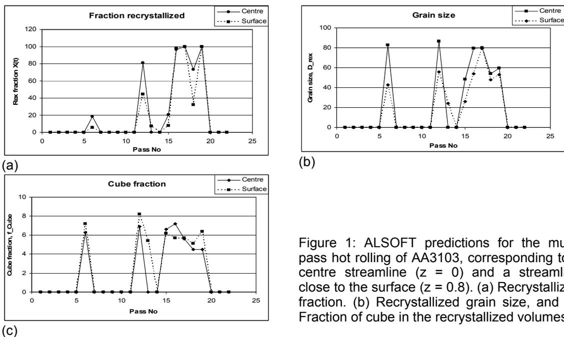
Figure 1: ALSOFT predictions for the multi-pass hot rolling of AA3103, corresponding to a centre streamline ( $z = 0$ ) and a streamline close to the surface ( $z = 0.8$ ). (a) Recrystallized fraction. (b) Recrystallized grain size, and (c) Fraction of cube in the recrystallized volumes.
