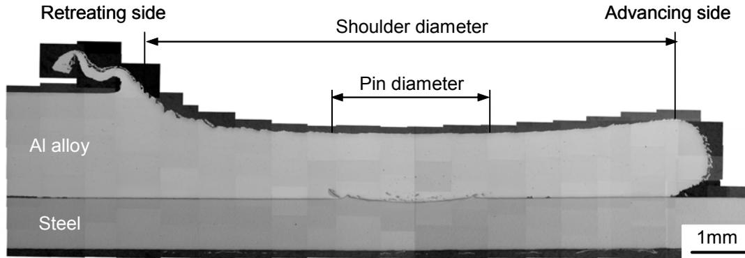
Figure 3: Optical micrograph of the transverse cross section of the steel / 6022 aluminum alloy joint fabricated at penetration depth : 2.1 mm.
