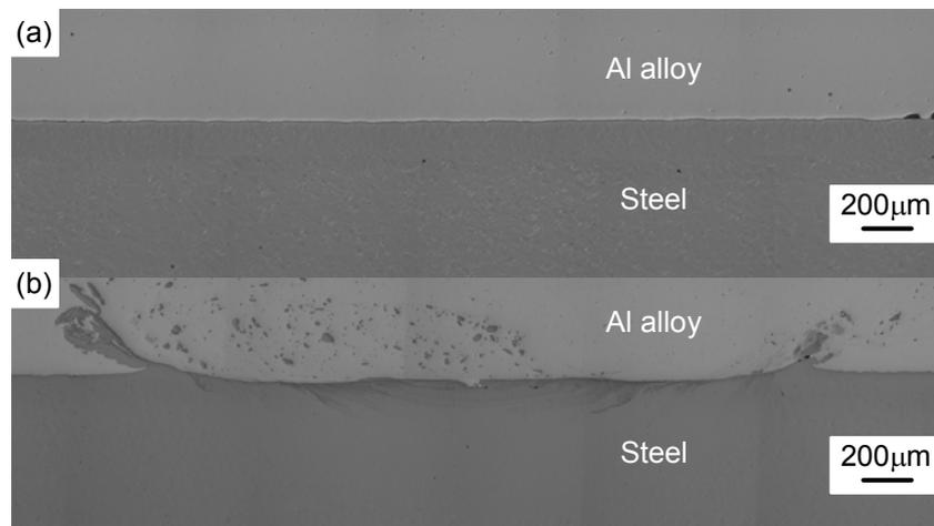
Figure 4: Optical micrographs of the cross section of steel / 6022 aluminum alloy interface. (a) penetration depth : 1.9 mm and (b) penetration depth : 2.1 mm.
