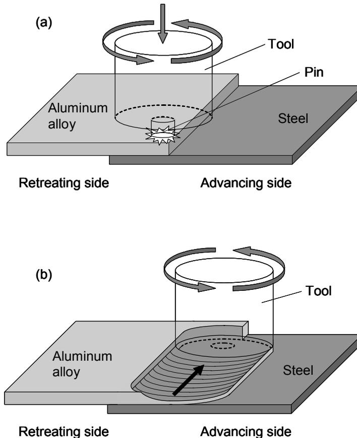
Figure 1: Friction stir welding process of steel / 6022 aluminum alloy joint. (a) A rotating tool is plunged into a aluminum alloy plate and (b) The tool is moved along the steel / aluminum interface.
