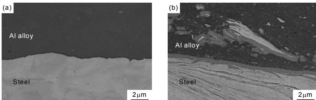
Figure 5: Back scattering electron images of steel / 6022 aluminum alloy interface. (a) penetration depth : 1.9 mm and (b) penetration depth : 2.1 mm.
