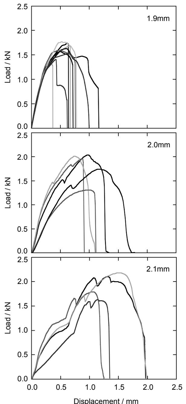
Figure 2: Load – displacement curves of the steel /6022 aluminum alloy joint.
