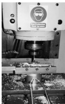
Figure 2.1: Tapping device and data acquisition apparatus.
