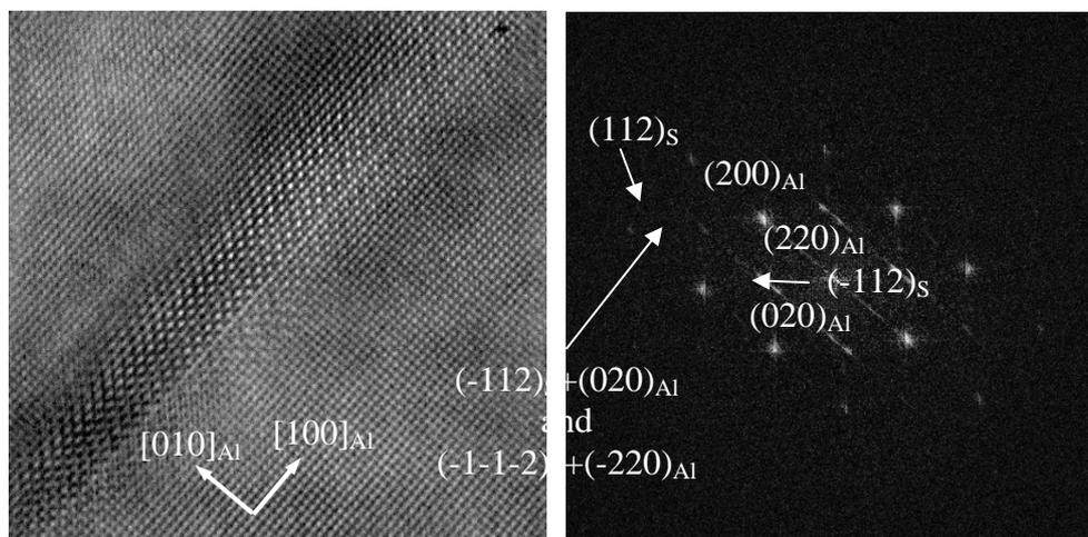
Figure 3: (a) S-phase particle viewed along the  $[100]$ . (b) corresponding FFT spectrum.
