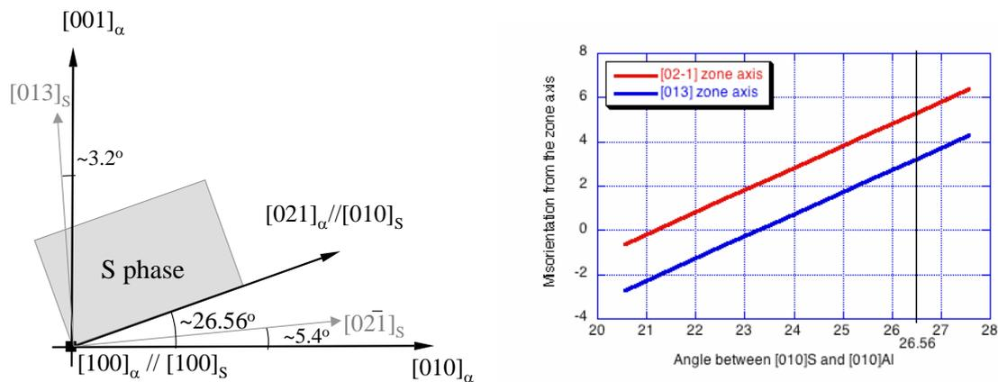
Figure 2: (a) Schematic of orientation relationship of the S-phase with Al matrix. (b) plot showing the misorientation of the  $[013]_S$  and  $[02-1]_S$  from the  $\langle 001 \rangle_{Al}$
