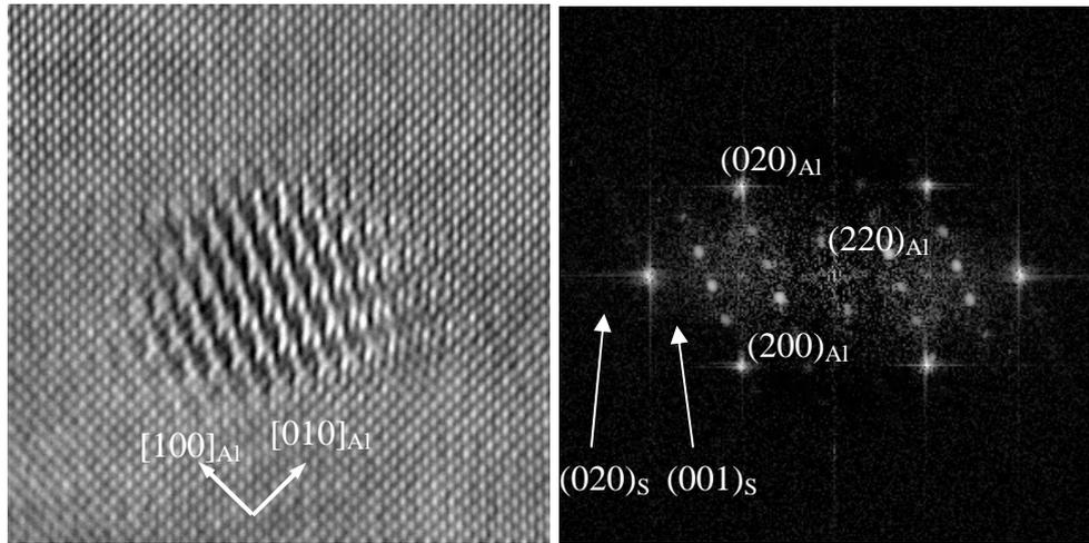
Figure 1: (a) S-phase particle viewed along the  $[100]_{Al}$ . (b) corresponding FFT spectrum.
