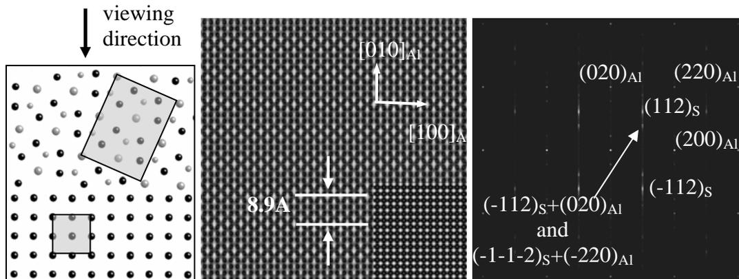
Figure 4: (a) A schematic of an overlay of Al and S-phase used in the computer simulation, (b) HRTEM simulations, for comparison an insert from the Al matrix is also shown, (c) Corresponding Fourier spectrum.
