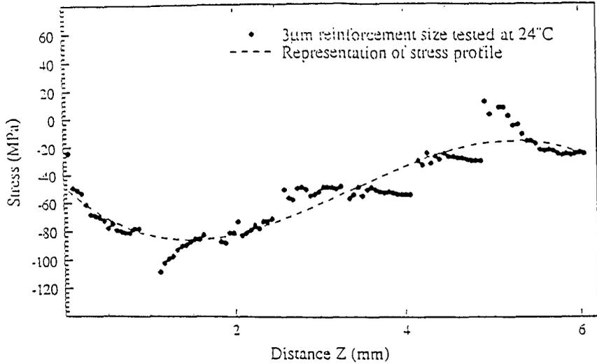
Figure 5.  $\sigma_x$  (residual stress in the x direction) vs. Z (hole depth), for the  $3\mu\text{m}$  reinforced composite to the specimen centre.
