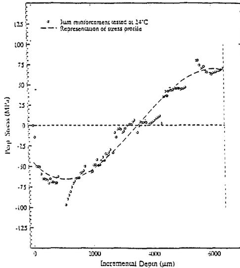
Figure 6.  $\sigma_x$  (residual stresses in the x direction) vs. Z (hole depth), for the  $3\mu\text{m}$  reinforced composite to the specimen centre. This figure gives the combination of both blind-hole drilling data and back face strain gauge information.
