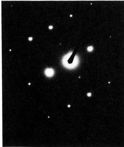
Figure 4: Selected area diffraction pattern illustrating presence of  $\delta'$  in solution treated Al-Cu-Mg-Li reinforced with 5 v/o  $\text{SiC}_w$ .
