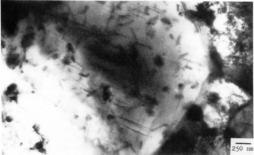
Figure 6: Transmission electron micrograph illustrating  $S'$  precipitation in Al-Cu-Mg-Li reinforced with 5 aged for 512 hrs at 100°C.
