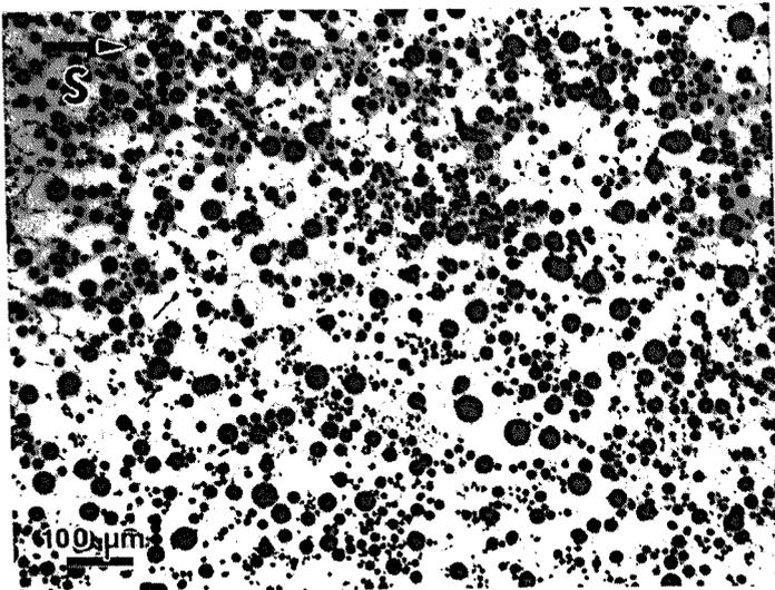
Figure 6. Optical micrograph of a directionally solidified specimen of Comral 90F composite at a furnace travel rate of  $\approx 100 \mu\text{m}\cdot\text{s}^{-1}$ .
