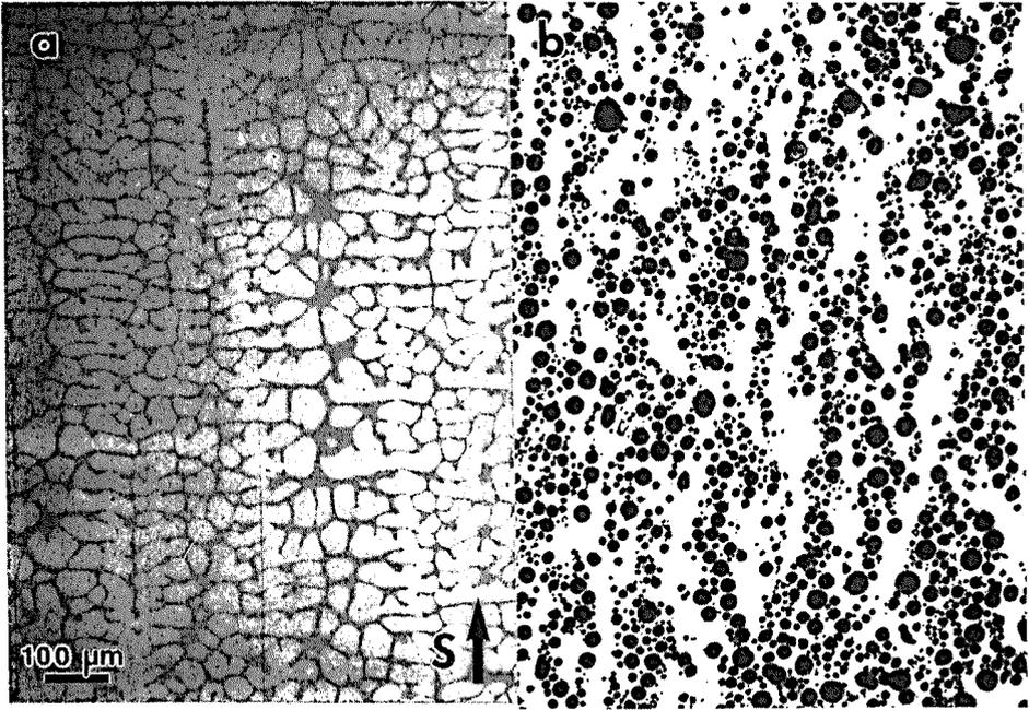
Figure 5. Optical micrographs of directionally solidified specimens of (a) an AA603 alloy, and (b) Comral 90F composite at furnace travel rate  $15 \mu\text{m}\cdot\text{s}^{-1}$ .
