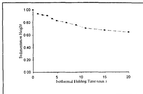
Figure 1. Sedimentation height plotted as a function of holding time for tube samples.
