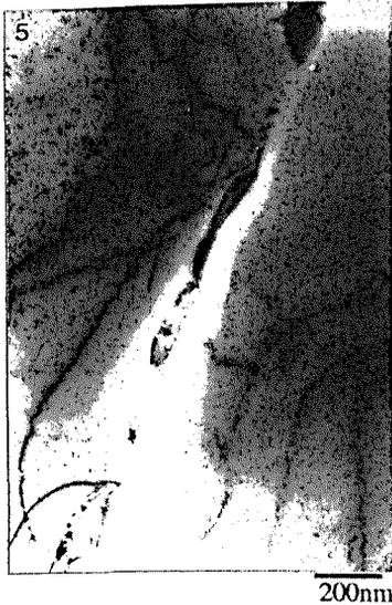
Figure 5. High aspect ratio I-phase particles in LV329 after SHT.
