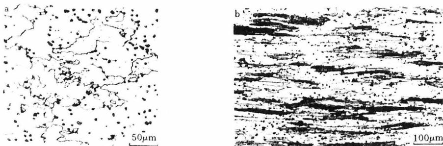
Figure 1. Optical microstructure of alloy 7A55
