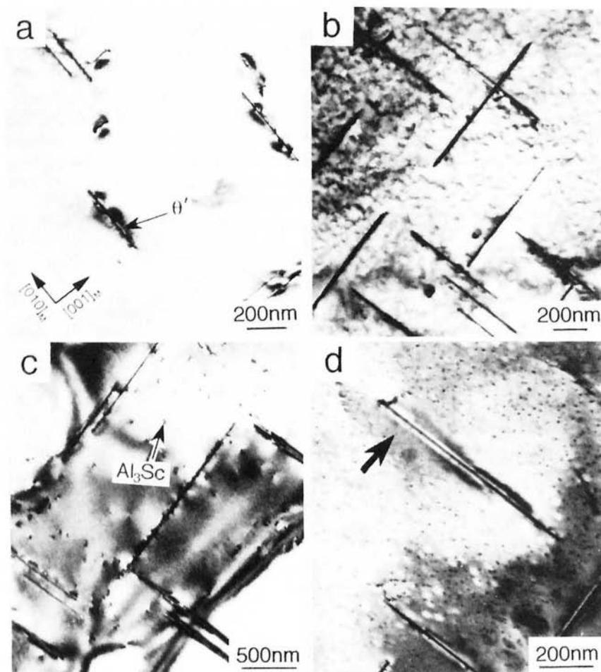
Fig.2 Transmission electron micrographs of Al-Cu-Sc alloy aged at 573K. Aging time is: (a)  $1.2 \times 10^3$  s, (b)  $6 \times 10^3$  s, (c)  $6 \times 10^4$  s, (d)  $6 \times 10^5$  s. Electron beam is parallel to  $[100]$  of the matrix.
