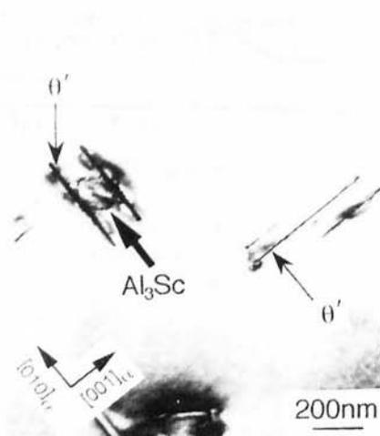
Fig.4 TEM image showing heterogeneous  $\theta'$  precipitation on the  $\text{Al}_3\text{Sc}$  particle which have existed before aging in the Al-Cu-Sc alloy aged 573K for  $1.2 \times 10^3$  s. Electron beam direction is parallel to  $[100]$  of the matrix.
