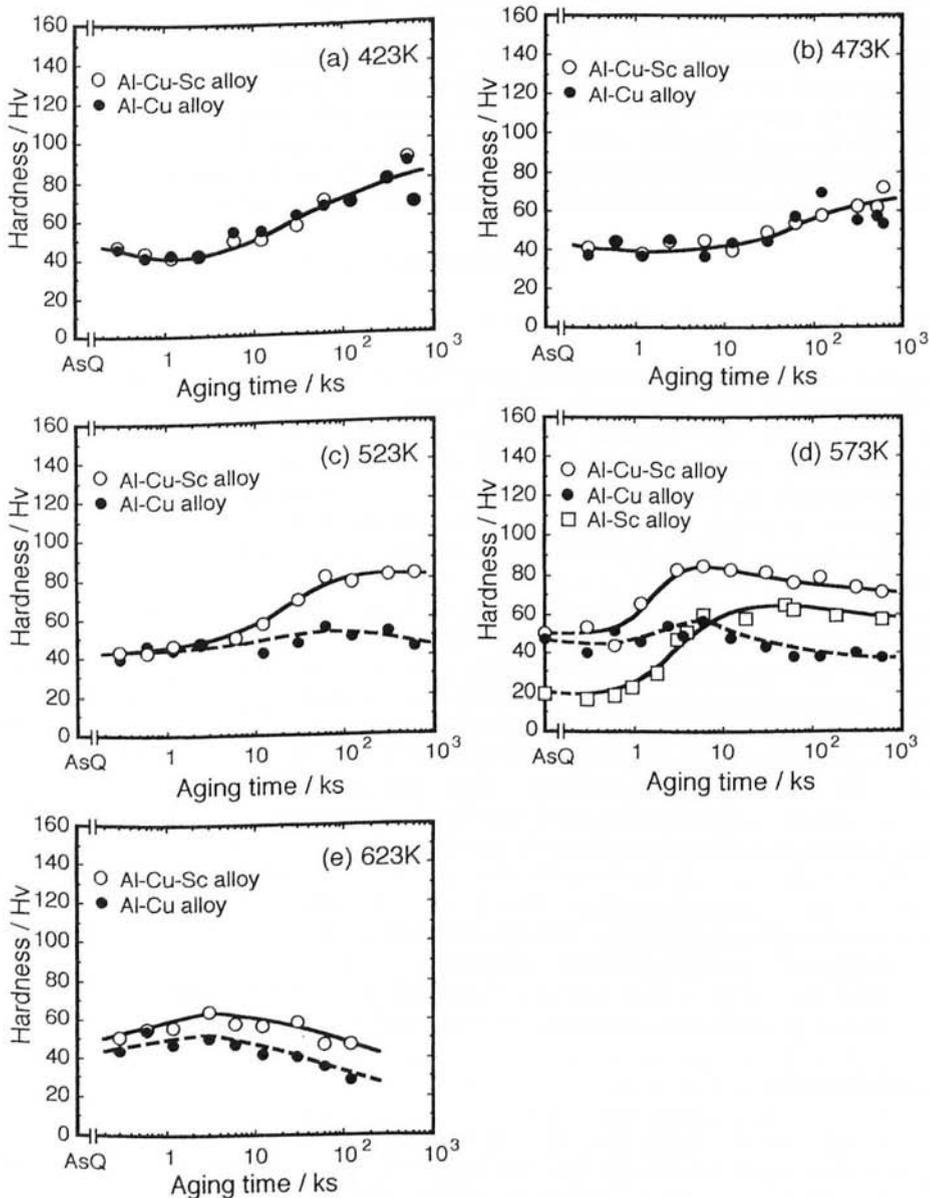
Fig.1 Age-hardening curves of Al-Cu-Sc alloy, Al-Cu alloy and Al-Sc alloy aged at : (a) 423K, (b) 473K, (c) 523K, (d) 573K and (e) 623K.
