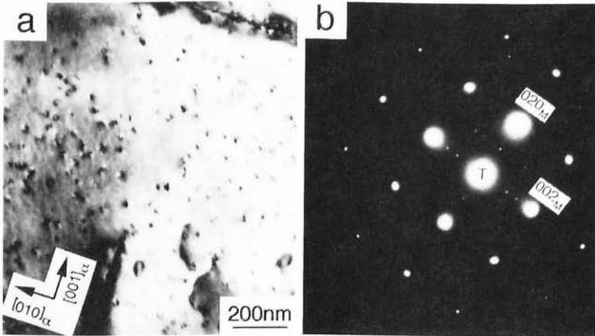
Fig.3 TEM image and selected area diffraction pattern of Al-Cu-Sc alloy aged at 623K for  $3 \times 10^3 \text{s}$ . Electron beam is parallel to  $[100]$  of the matrix.
