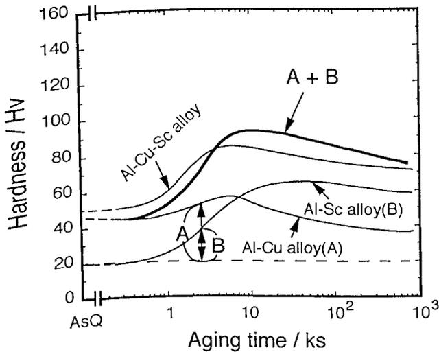
Fig.5 Comparison of the age-hardening curve of Al-Cu-Sc alloy with the sum of the age-hardening curves of Al-Cu alloy and Al-Sc alloy aged at 573K.
