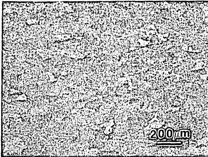
Figure 5. Photomicrograph showing as-deformed microstructure (true strain of 0.8) with complete recrystallization, 500 C and 20 s<sup>-1</sup>.
