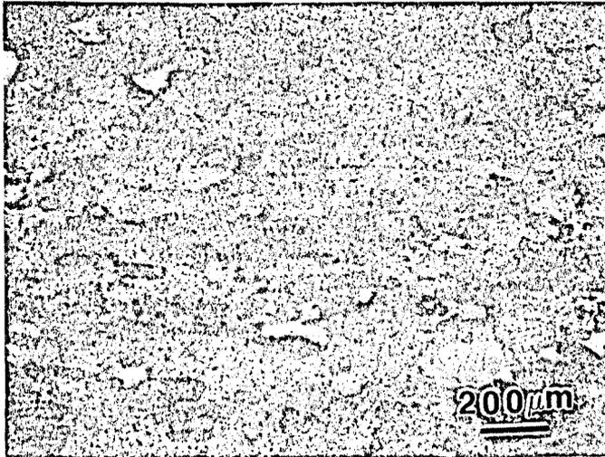
Figure 4. Photomicrograph showing as-deformed microstructure (true strain of 0.8) with partial recrystallization, 450 C and  $20 \text{ s}^{-1}$ .
