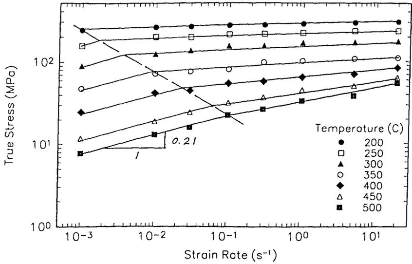
Figure 9. Effect of strain rate on flow stress for Al 6061 at a true strain of 0.5.
