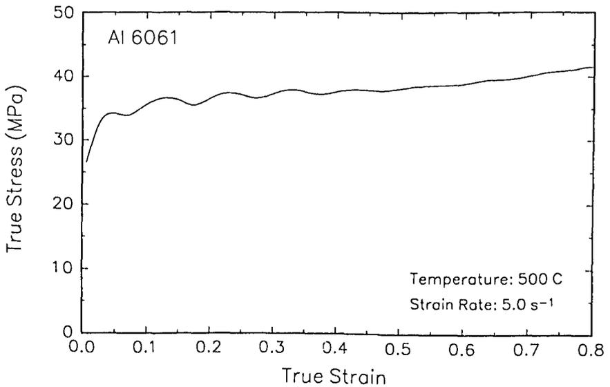
Figure 6. Flow curve showing repeated hardening and softening at 500 C and 5 s<sup>-1</sup>.
