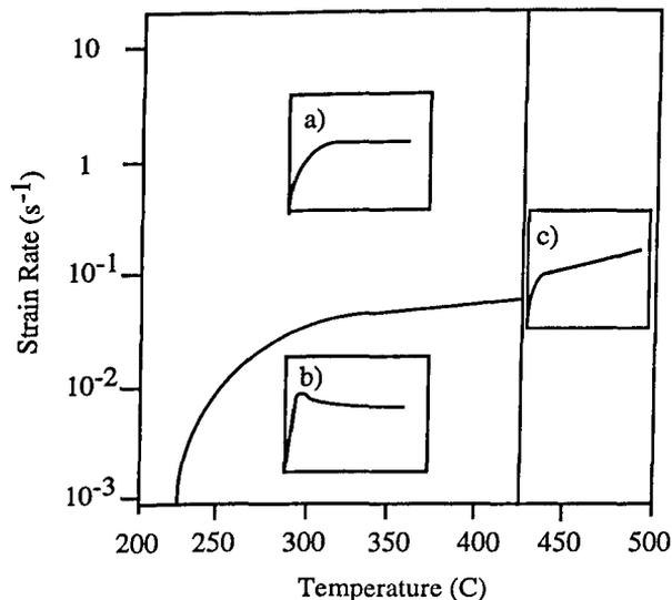
Figure 2. A schematic of the three types of flow curves as function of temperature and strain rate.
