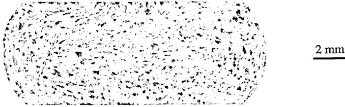
Figure 7. Example of relatively uniform flow, true strain of 0.8, 500 C and  $0.001\text{ s}^{-1}$ .
