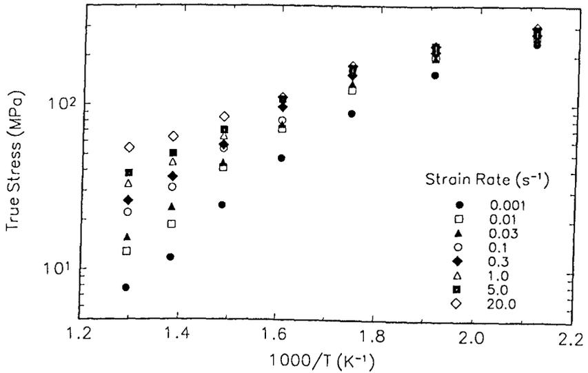
Figure 10. Effect of temperature on flow stress for Al 6061 at a true strain of 0.5.
