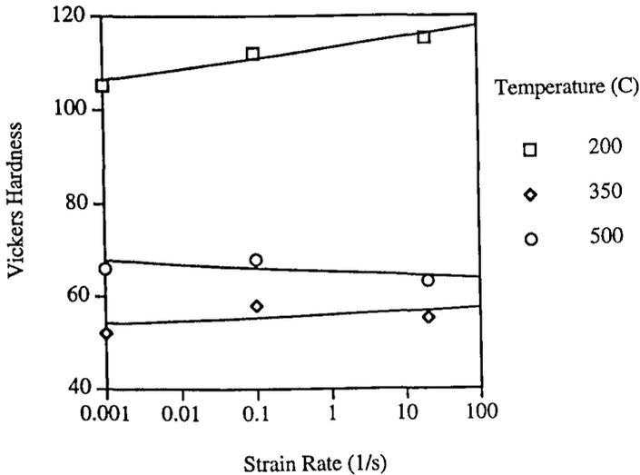
Figure 8. Room temperature hardness values on the specimens deformed at various temperatures and strain rates.
