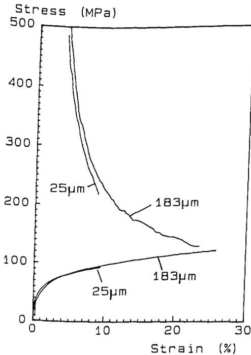
Figure 5. The lower curves show the stress-strain curves for soft annealed AA8111 foil at two different gauges. The upper curves give the derivative of stress upon strain.
