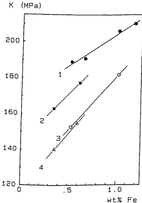
Figure 7. Plot of  $K$  in the Ludwik-Hollomon equation versus the alloy content of iron.
