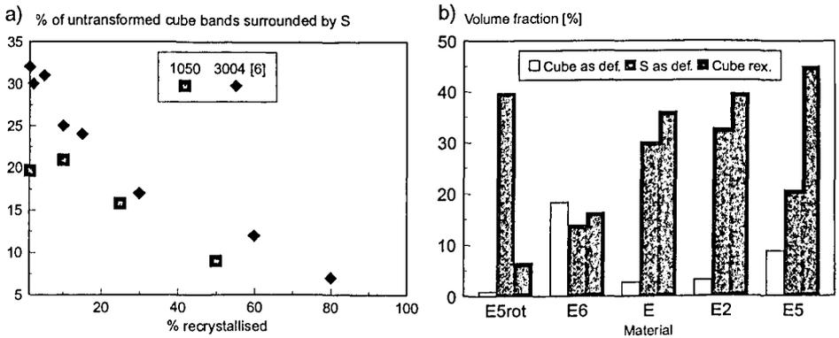
Figure 4. a) fraction of untransformed cube bands with  $40^\circ\langle 111 \rangle$  boundary to neighbour,  $\epsilon=2$ ,  $Z=10^{14}$ , b) fraction of recrystallised cube as a function of amount of S and cube after deformation,  $\epsilon=2$ ,  $Z=10^{14}$ , [10]
