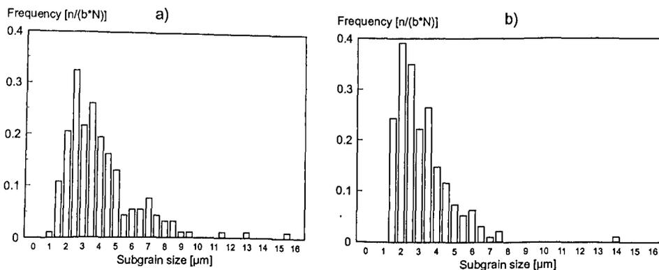
Figure 2. Subgrain size distributions: a) cube, b) others,  $\epsilon=2$ ,  $Z=10^{14}$  ( $\xi=0.6$ ,  $300^\circ\text{C}$ )
