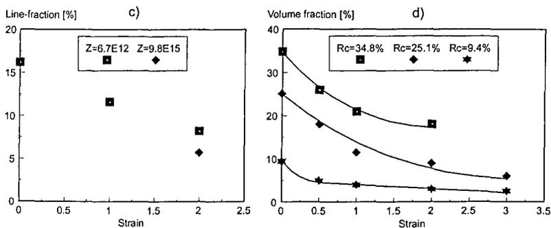
Figure 1. c) Line fraction of cube, EBSP, d) Volume fraction of cube, X-ray ( $Z=6.7 \cdot 10^{12}$ ,  $R_c$ =initial cube fraction)
