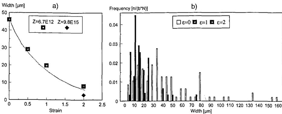
Figure 1. a) average cube band width, b) distribution of band widths ( $Z=6.7 \cdot 10^{12}$ ,  $\xi=2.5$ ,  $400^\circ\text{C}$ )
