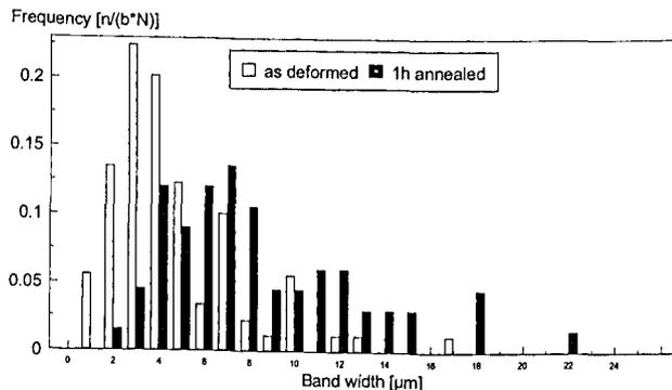
Figure 5. Distribution of cube band widths, as deformed and 1h annealed at  $300^\circ\text{C}$ ,  $\epsilon=2$ ,  $Z=10^{14}$  ( $\xi=0.6$ ,  $300^\circ\text{C}$ )
