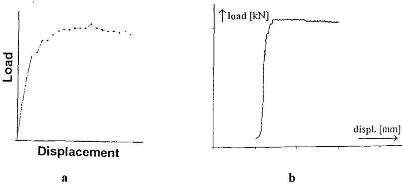
Fig.1. Typical extrusion load - displacement curve, a. direct, b. indirect extrusion
