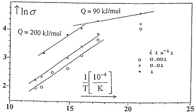
Fig 6. To the calculation of the activation energy
