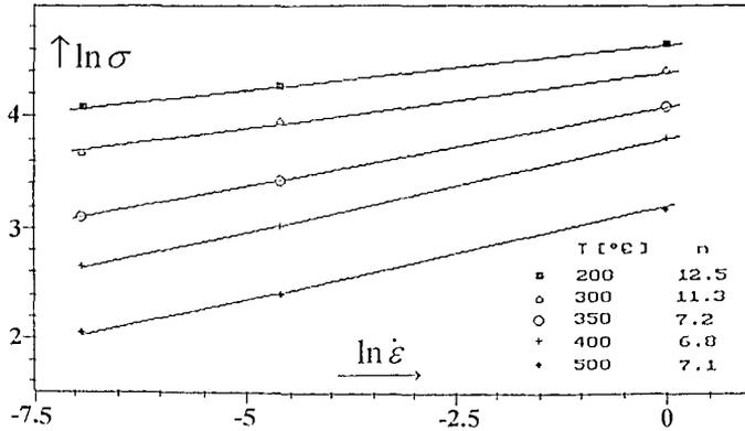
Fig. 5. Strain rate dependence of the flow stress
