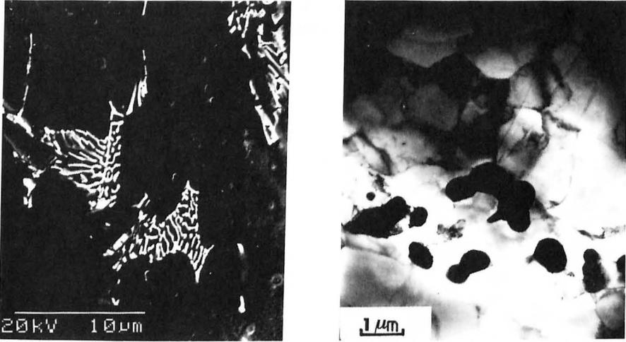
Fig. 1. (a) SEM micrograph of the as-cast material showing dendrite-like morphology particles. (b) TEM of the same material showing both particles and dislocation arrangements.
