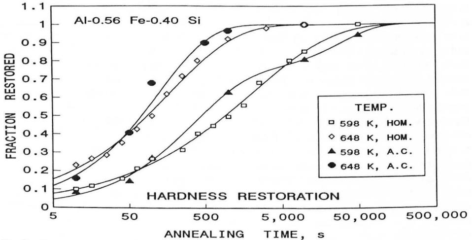
Fig.3. Change of the fraction restored with annealing time at two different temperatures.
