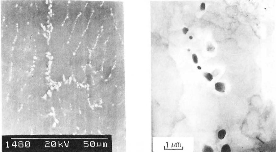
Fig. 2. (a) SEM micrograph of the homogenized alloy showing the resulting particle distribution. (b) TEM micrograph of the same alloy showing significant changes in the dislocation substructure.
