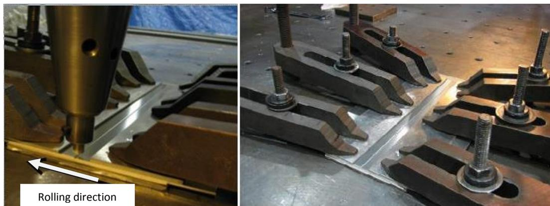
Figure 3. FSW tailor welded coupons development.
