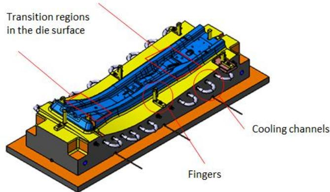
Figure 8. Tool CAD of tailored thickness die.
