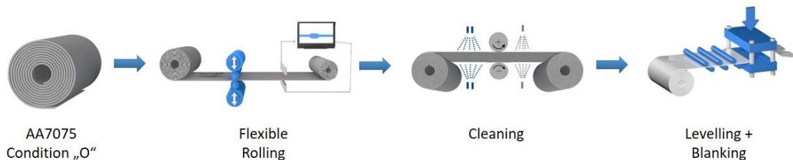
Figure 2. Process chain of flexible rolling
