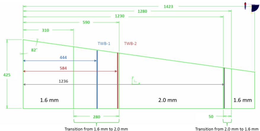
Figure 9. Blank dimensions for tailor rolled/welded blanks.
