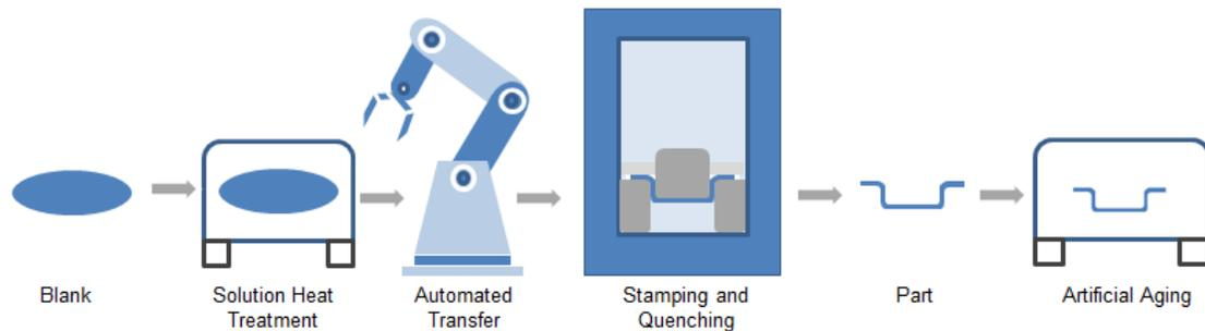
Figure 10. Schematic of the hot stamping process.
