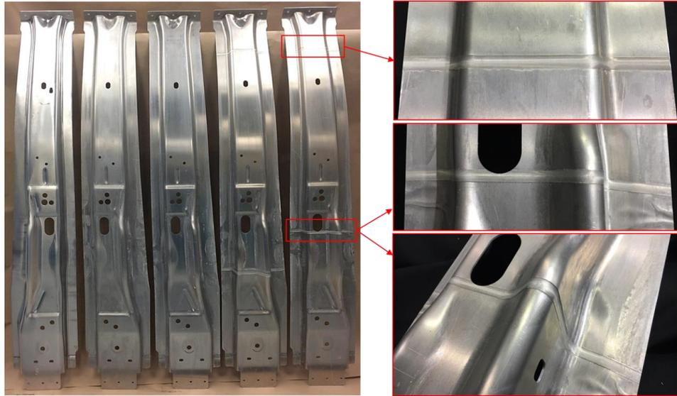
Figure 11. 6xxx production B-pillar compared to hot stamped B-pillars from AA7075; a) 6xxx; b) 7xxx c) TRB, d) TWB-1, e) TWB-2.
