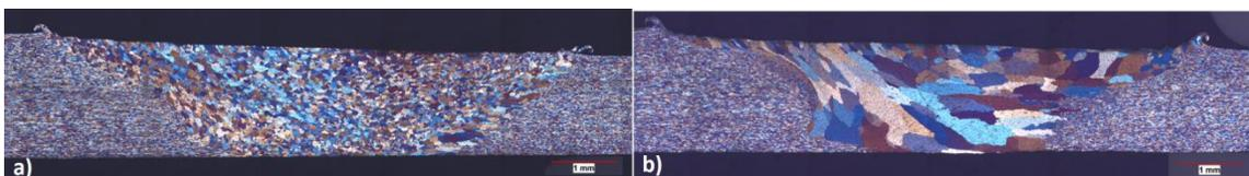
Figure 6. Microstructural analysis after high temperature heat cycle; a) competitive grain growth; b) abnormal grain growth.
