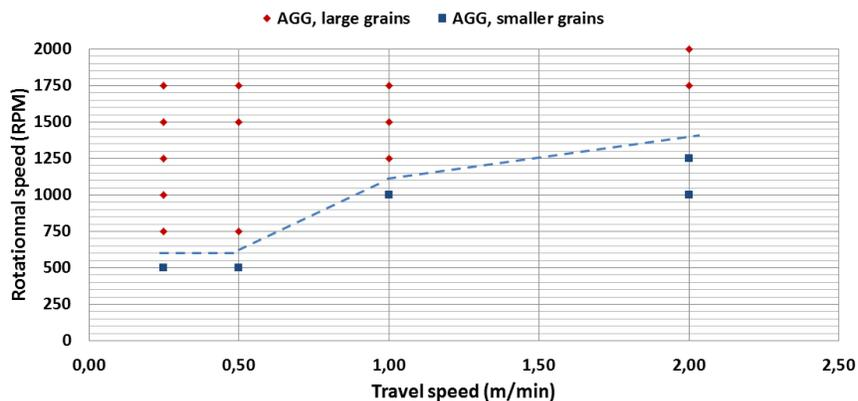
Figure 5. Abnormal grain growth behavior upon various FSW process conditions.
