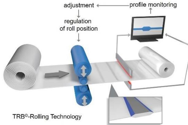
Figure 1. Principle of the flexible rolling process
