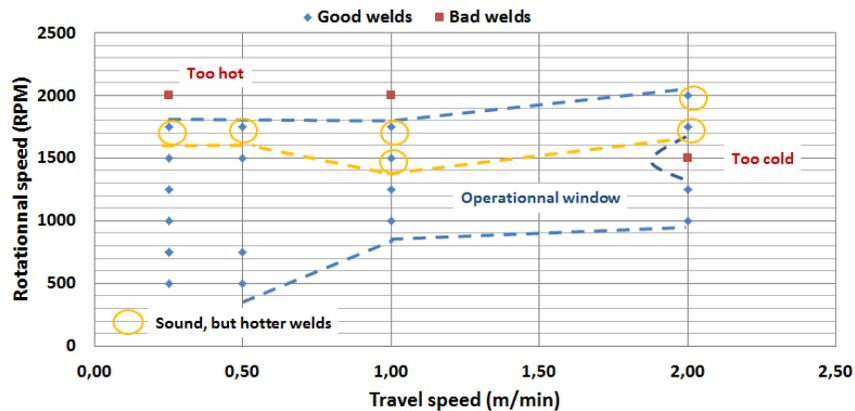
Figure 4. Process window determination for cup shoulder design FSW tool.
