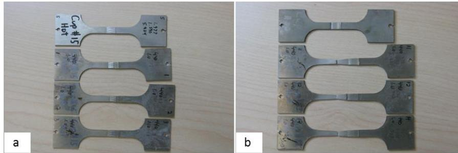
Figure 7. Hot tensile testing behavior; a) abnormal grain growth; b) competitive grain growth.
