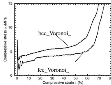
Figure 2. Compressive stress-strain curves of bcc\_Voronoi\_[001] and fcc\_Voronoi\_[001]
