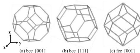
Figure 1. Images of unit cells of bcc\_Voronoi\_(a),(b) and fcc\_Voronoi\_(c)
