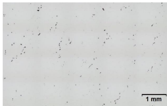
Figure 2. Assembly of micrographs of the cast and homogenized material. Assemblies with total areas ranging from 20 to 30 mm 2 for each specimen were used for the evaluation of voids.
