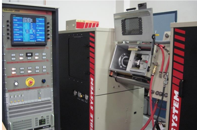
Figure 1. Overview of Gleeble 3800 thermo-mechanical physical simulator system
