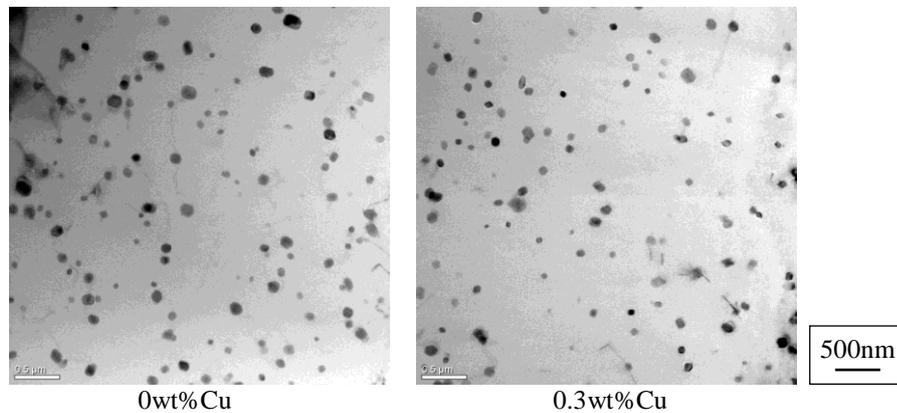
Figure 4. Distribution of fine precipitates in 0wt%Cu and 0.3wt%Cu after brazing heat treatment
