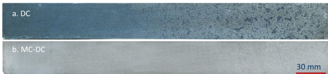
Figure 1. a) Coarse grain structure of conventional DC billet of an A4xxx alloy of 650 mm diameter with 2 ppt AlTiB grain refiner and b) fine and uniform grains in MC-DC billet without grain refiner addition.
