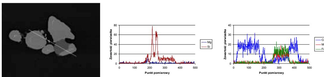
Fig. 3 The linear analysis of chemical composition running through the precipitates of copper, iron,  $Mg_2Si$  and Si in as-cast sample no. 3.
