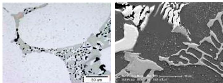
b. The intermetallic phases in sample no. 4.4 (Mg-0,8%, Si-1%, Mg/Si=8, cooling rate of 0,5K/s).
