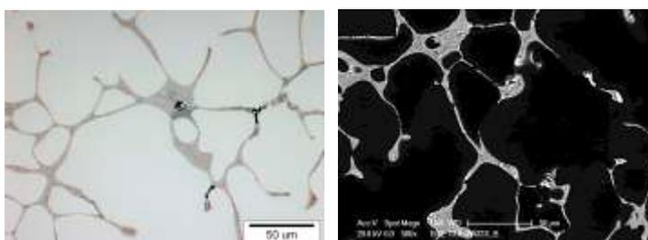
a. The intermetallic phases in sample (SC) taken from the centre of as-cast ingot.
