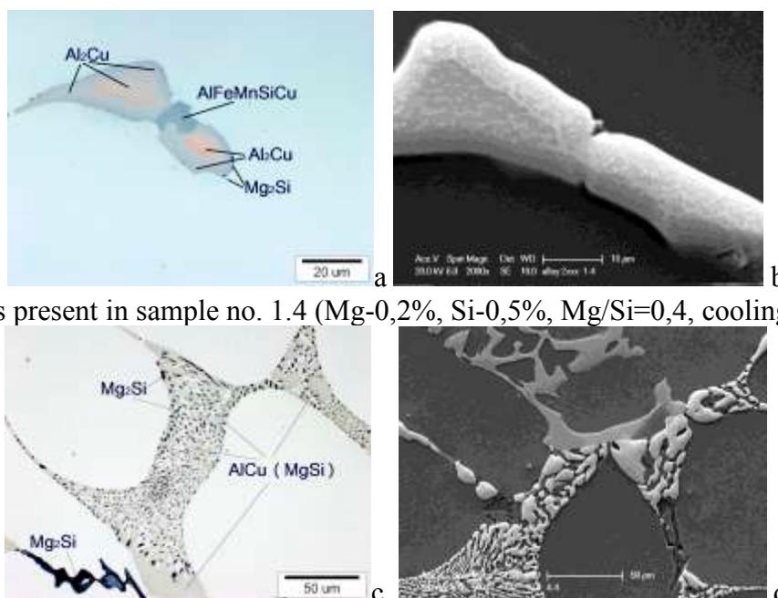
1a.  $AlCu$  phases present in sample no. 1.4 (Mg-0,2%, Si-0,5%, Mg/Si=0,4, cooling rate of 0,5K/s ).
