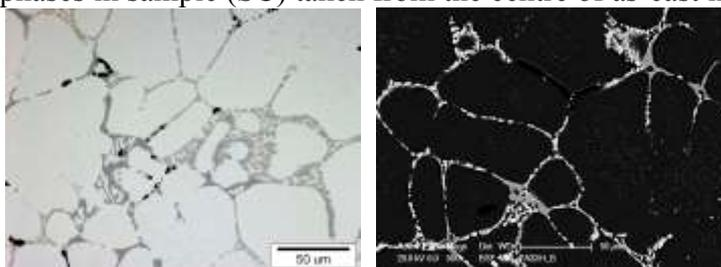
b. The intermetallic phases in sample (SH) taken from the centre of ingot after homogenisation.
