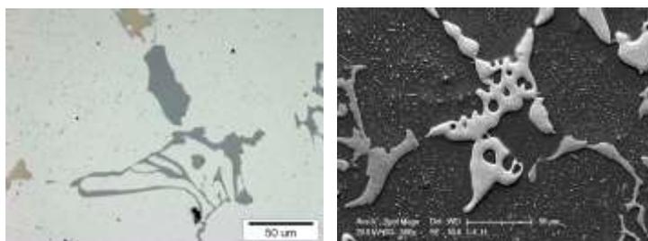
a. The intermetallic phases in sample no. 1.4 (Mg-0,2%, Si-0,5%, Mg/Si=0,4, cooling rate of 0,5K/s).
