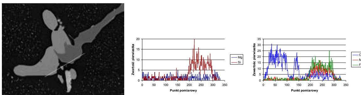
Fig. 5. The linear analysis of chemical composition running through the precipitates of copper and iron in sample no. 3 after homogenising treatment.
