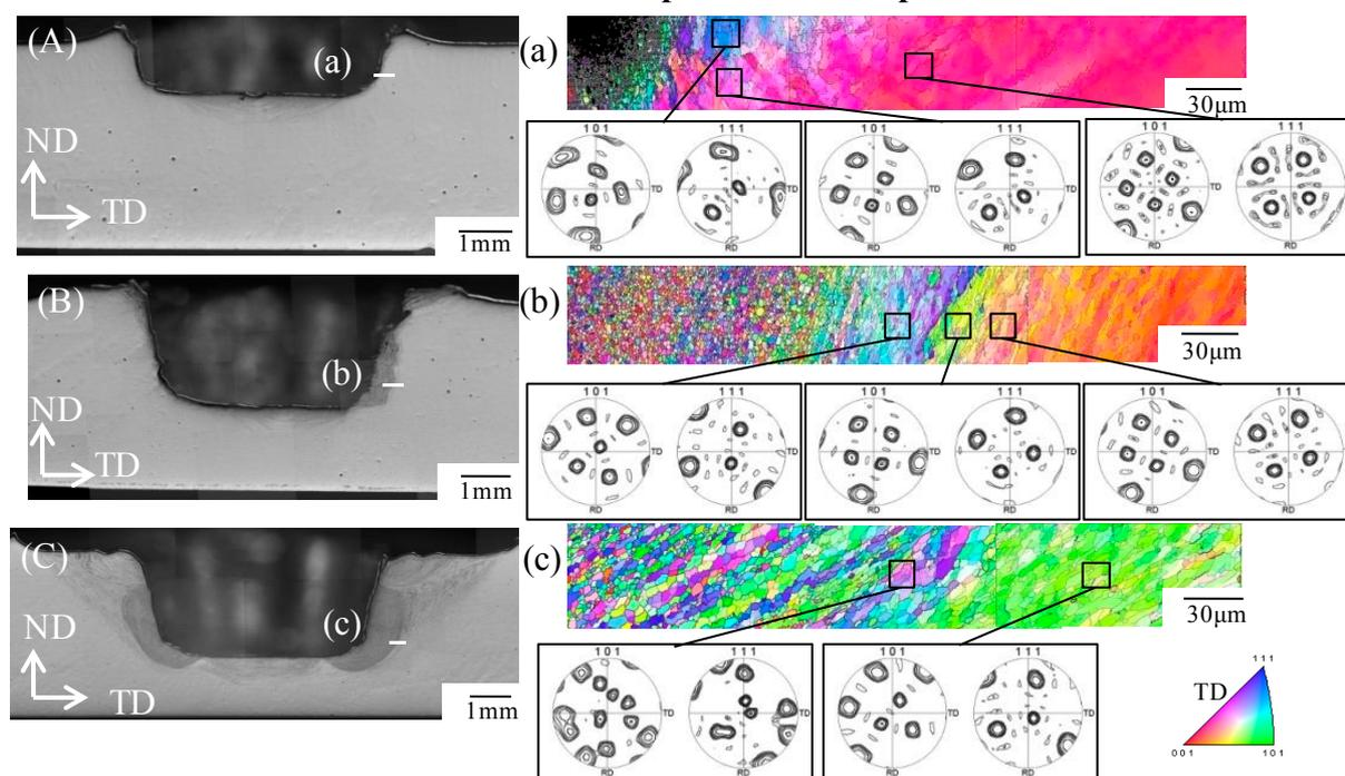
Fig. 2 Cross sections of friction stir spot welded high purity aluminum samples.
