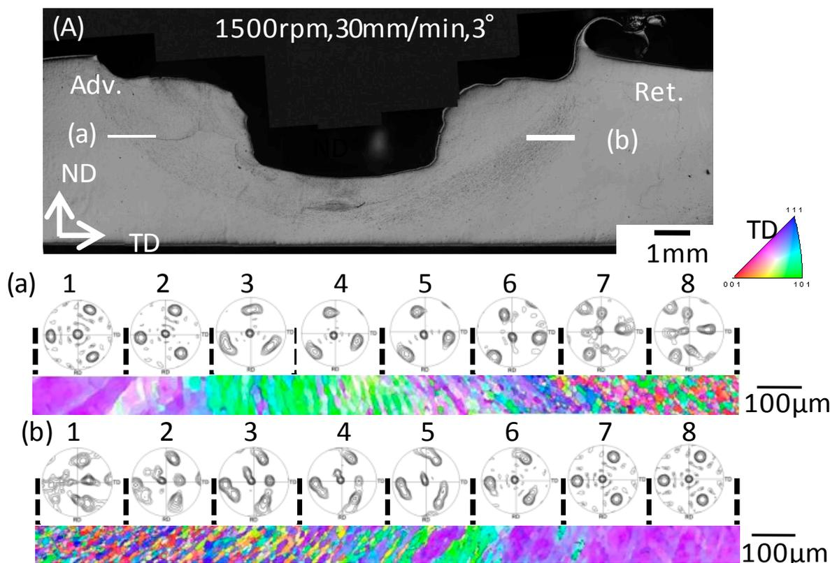
Fig.3 Cross sections of friction stir welded high purity aluminum samples.
