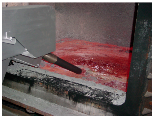
Fig. 9 PHD-50 in operation generates little turbulence
