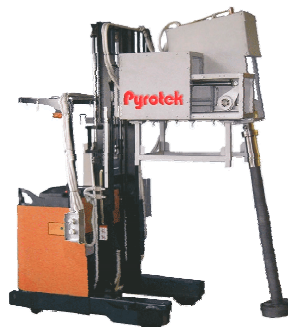
Fig. 3 PHD-50 unit injecting bi-gas with rotary nozzle
