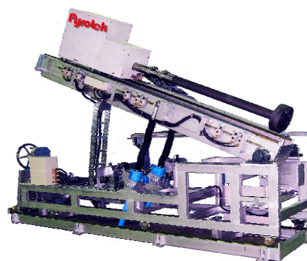
Fig. 4 HD-2000 System injecting bi-gas of chlorine and nitrogen gas
