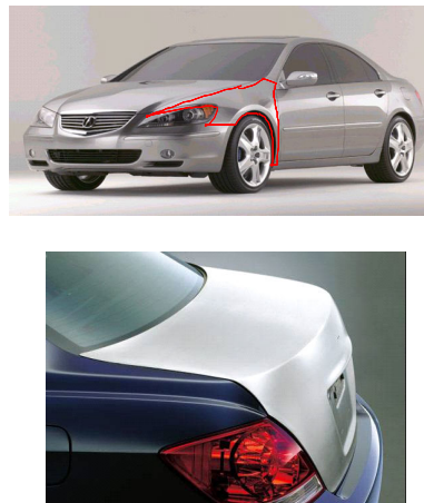
Fig.17 Fender and trunk-lid of Honda Legend produced by high speed blow forming.
