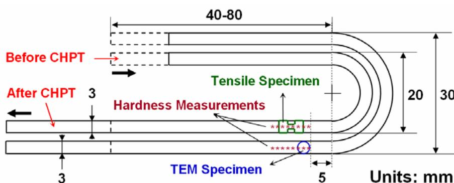
Fig. 3. Dimensions of U-shaped samples including positions for microhardness measurements and locations for tensile specimen and TEM disc.
