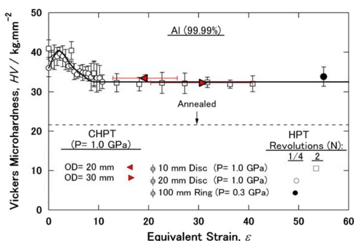
Fig. 4. Hardness value for CHPT plotted against equivalent strain in graph reported earlier using conventional HPT for disc and ring specimens of Al [8].
