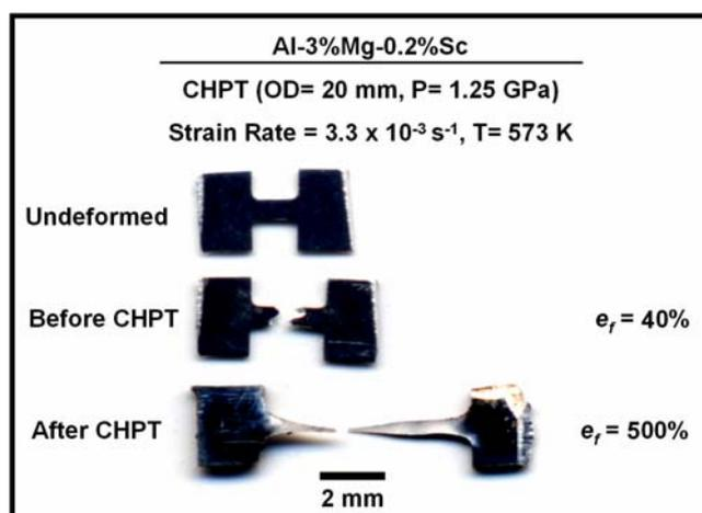
Fig. 8. Appearance of tensile specimens after pulling to failure at 573 K before and after processing by CHPT. Undeformed specimen is also included.
