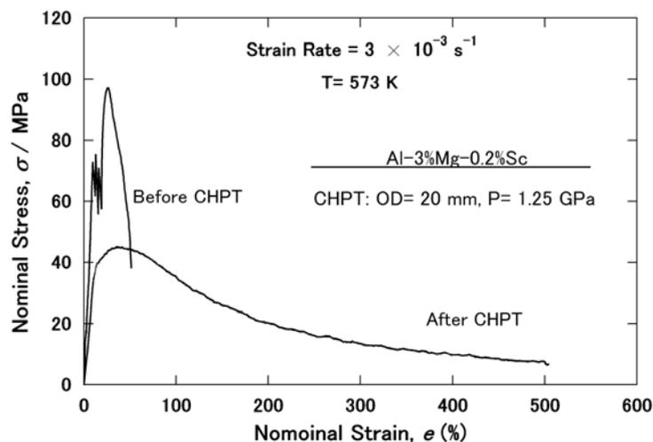
Fig. 7. Nominal stress versus nominal strain curves of Al-3%Mg-0.2%Sc before and after processing by CHPT.
