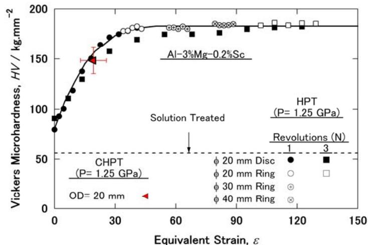
Fig. 6. Hardness value for CHPT plotted against equivalent strain in graph reported earlier using conventional HPT for disc and ring specimens of Al-3%Mg-0.2%Sc [13].
