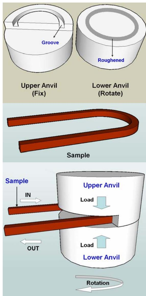
Fig. 1. Schematic illustration of CHPT.
