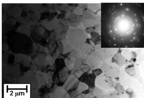
Fig. 5. Bright-field TEM micrograph and SAED pattern of Al after processing with CHPT.
