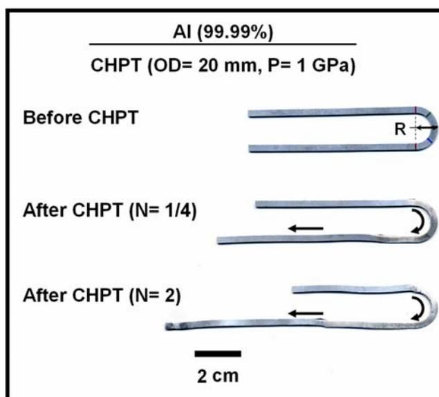
Fig. 2. Appearance of U-shaped Al samples with  $OD= 20$  mm before and after CHPT for 1/4 and 2 revolutions.
