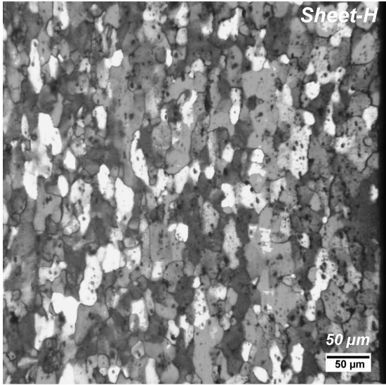
Fig 1. Optical images taken in the longitudinal sections of the sheets showing the grain structures. The RD is vertical.
